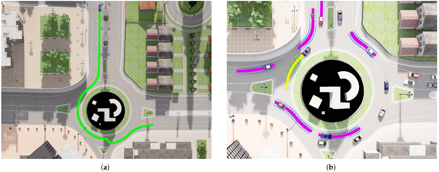
Figure 5. Experimental setup in Town 3. (a) Ego vehicle's fixed global route ( \approx 150 m): straight approach, roundabout entry with a lane change, and a designated exit branch (green path). (b) Safety Potential computation: yellow points and green cells denote the ego vehicle's planned path and occupancy cells, while purple points and blue cells denote surrounding vehicles' predicted trajectories and occupancy cells; time-weighted overlaps between these cells yield the per-frame SP. The same global route and traffic protocol are used for all experiments to ensure comparability.
