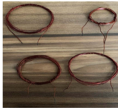
Figure 11. Coils having different turns ( N ) and thickness.
