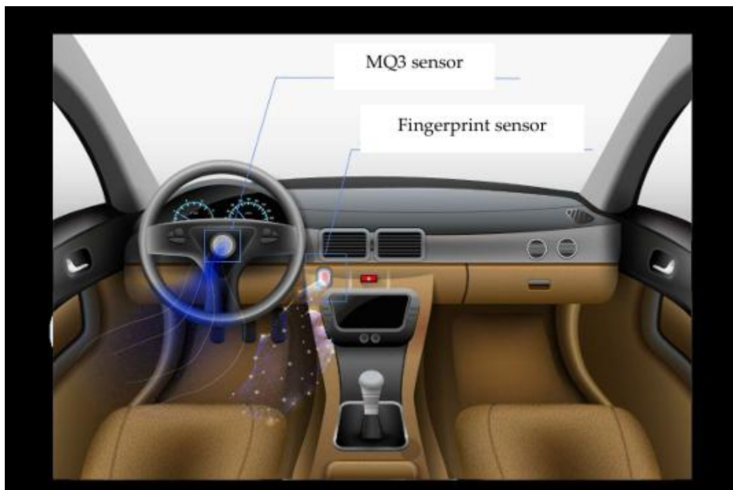
Figure 9. Possible placement of the fingerprint and the MQ3 sensors within a car.
