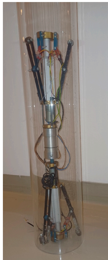
Figure 7. Fabricated ASDIR hardware prototype mounted inside a transparent pipe for planned experimental validation.
