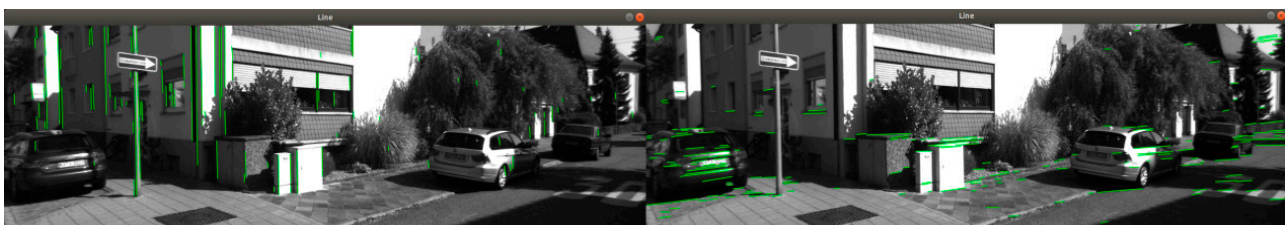
(a) Grouping of line features at 90\text{--}100^\circ intervals (b) Grouping of line features at 10\text{--}20^\circ intervals
