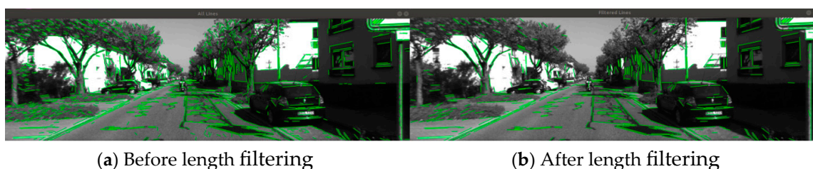
Figure 2. Comparison of adaptive length filtering effects.
