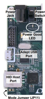
Figure 14. Starting up the Atlys FPGA development board [19].
