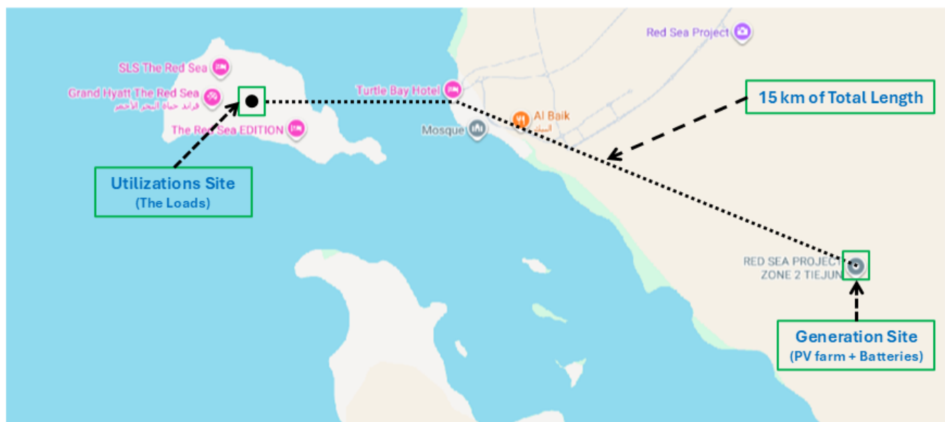
Figure 13. Distribution lines connecting the solar farm and BESS with the utilization site.
