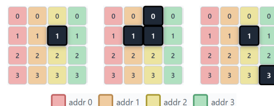
Figure 1. Physical distinction between SCU (left, single particle/single bit flip), MCU-3 (center, single particle/multiple adjacent flips via lateral charge diffusion), and coincident SCU (right, two independent strikes producing a non-adjacent bit pair indistinguishable from MCU on the basis of logical coordinates alone). Black boxes denote SRAM cells affected by bit upsets.
