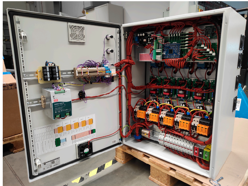
Figure 12. Laboratory prototype of the developed 75 kW 5P-TSBB converter.
