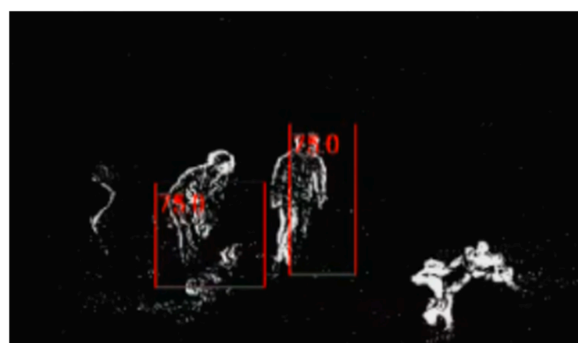
Figure 6. DVS-based person detection result in an indoor environment. The event-derived image emphasizes the moving person’s contour while suppressing static background information. Using the Faster R-CNN-style detector with a lightweight backbone, the proposed implementation achieves 92 ms processing latency on an Exynos 7570 mobile processor. The red rectangular boxes indicate the bounding boxes predicted by the detection network to localize the persons.
