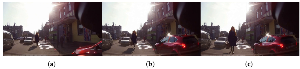
Figure 9. Three frames from a generated video clip illustrating depth drift: (a) at t = 1 , the pedestrian approaching the ego vehicle appears at a plausible distance; (b) at t = 3 , anomalous scale growth becomes apparent as the pedestrian enlarges rapidly; (c) at t = 5 , the pedestrian towers above the reference SUV visible on the right side.
