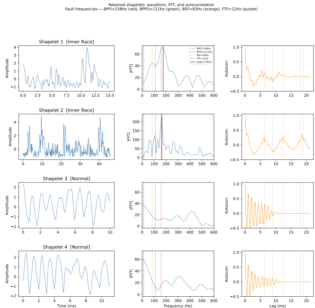
Figure 3. Retained shapelets from the best CWRU configuration (train+val, n_{\text{samp}} = 418 , max_shapelets = 8; four selected after self-similar removal). Left: shapelet waveform. Centre: FFT magnitude (dashed lines mark fault characteristic frequencies: BPFI = 158 Hz red, BPFO = 111 Hz green, BSF = 83 Hz orange, FTF = 12 Hz purple; solid black vertical line is the spectral peak). Right: normalised autocorrelation (dotted lines at expected inter-impact periods for each fault frequency). Shapelets 1–2 (Inner Race) have dominant spectral energy near BPFI; Shapelets 3–4 (Normal) capture high-frequency background texture at 900–930 Hz, inconsistent with any fault characteristic frequency.
