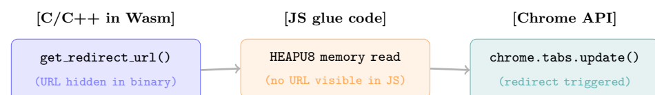
Figure 3. Data flow across the Wasm–JS–Chrome API boundary in the Forced Redirect scenario. The redirect target URL is encoded in the Wasm binary and never appears in JS source, rendering it invisible to JS-based static analyzers.
