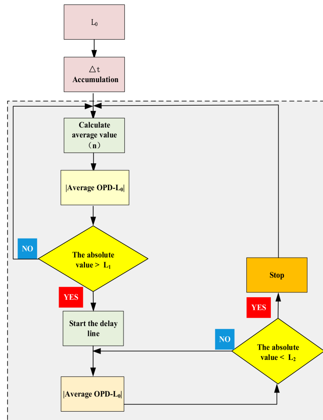
Figure 4. Flowchart of the optical fiber delay line control program.
