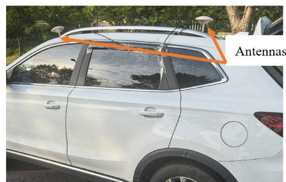
Figure 7. The picture of installation of the antennas.
