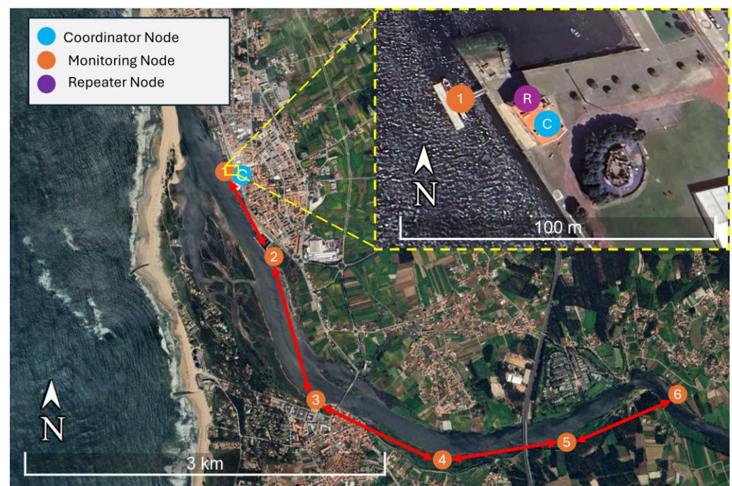
Figure 10. Temporary installation of the WSN in the Cávado estuary.
