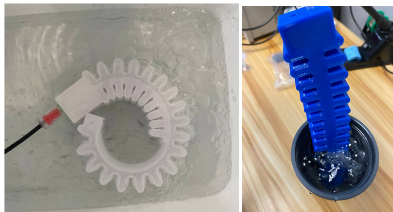
Figure 10. Bubble-leakage testing of the FFF-printed TPU pneumatic actuator during pressurization.
