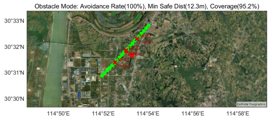
Figure 12. Trajectory comparison in geographic coordinates under the obstacle scenario. Red circles, crosses, and the star denote no-fly zones, their centres, and the ground station, respectively. The RRT* path circumvents all obstacles and converges rapidly toward the ideal trajectory, achieving 95.2% beam coverage.
