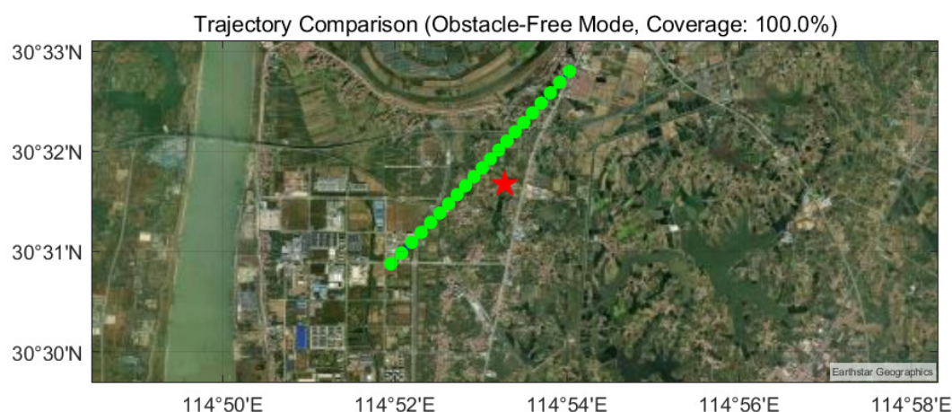
Figure 8. Trajectory comparison in geographic coordinates for the obstacle-free scenario. Green dots indicate UAV positions that fall within the radar beam; the red star marks the ground station. The ideal trajectory and the planned trajectory nearly overlap throughout the pass, with all points remaining within beam coverage.
