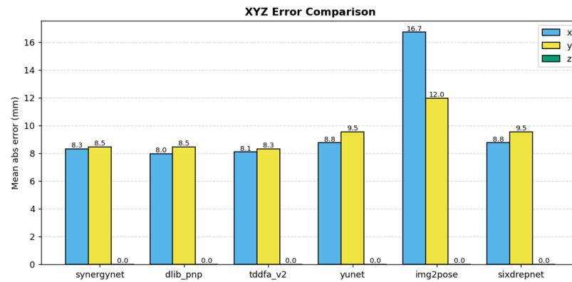
Figure 16. Decomposition of the 3D localization error into orthogonal the X-, Y-, and Z-axis spatial components, revealing anisotropic tracking characteristics.
