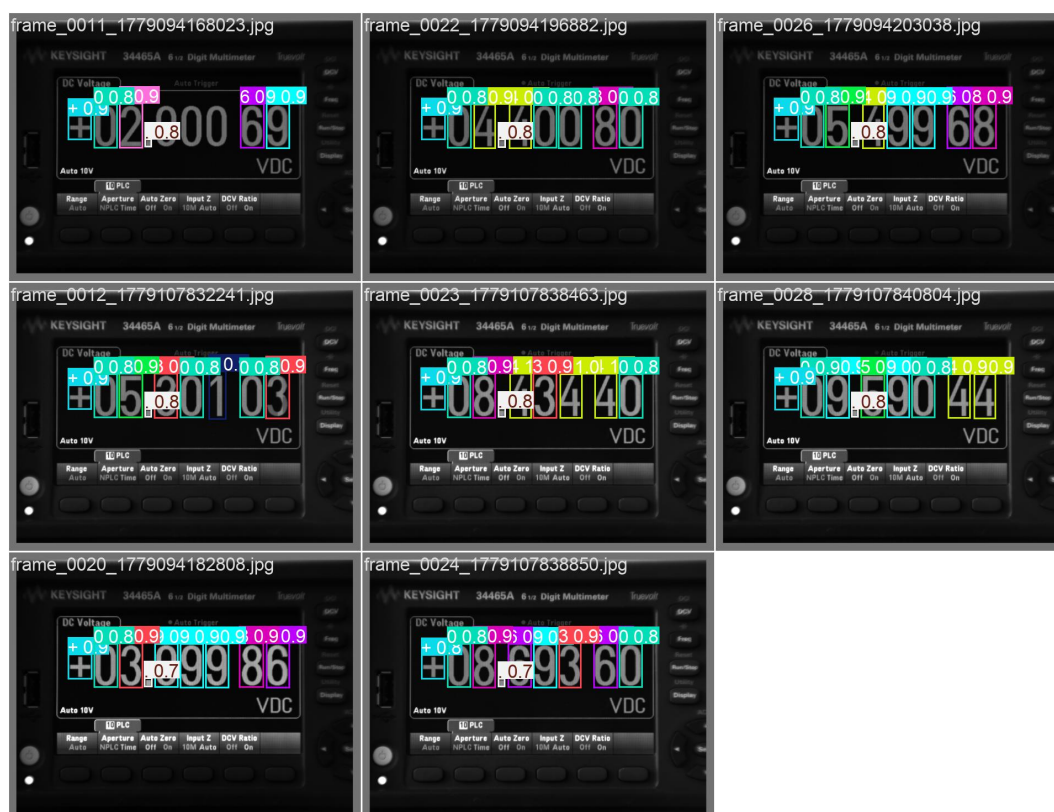
Figure 4. Example results of character detection on the multimeter display obtained using the trained YOLOv8s model.
