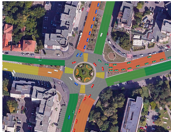
Figure 15. Simulation of the selected real-world intersection and AnyLogic density map. The satellite image is used as the geometric background, while the coloured road sections represent local traffic speed, ranging from red, approximately 5 km/h or lower, to green, approximately 50 km/h or higher.
