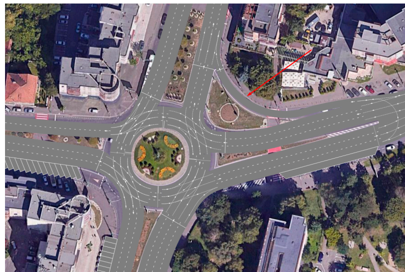
Figure 18. The addition of a right-turning vehicle lane. The red arrow indicates the added slip lane (bypass lane) for right-turning vehicles.
