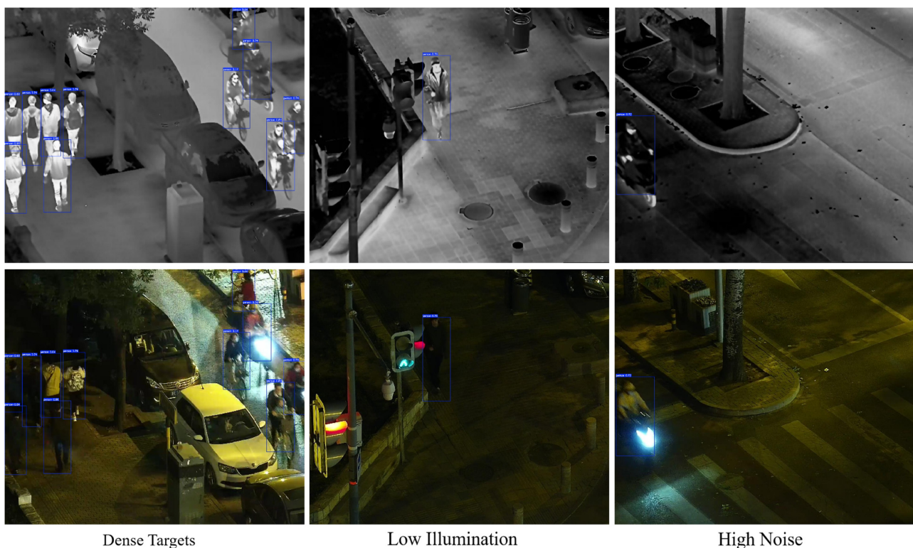
Figure 10. Visual detection results of the DMAC-Net architecture on the LLVIP dataset. Each column represents a different scene type: from left to right, high-noise, low-light, and dense target scenarios. Only containing one type of "person" category target, in the group of images, it is represented by blue detection boxes and labels.
