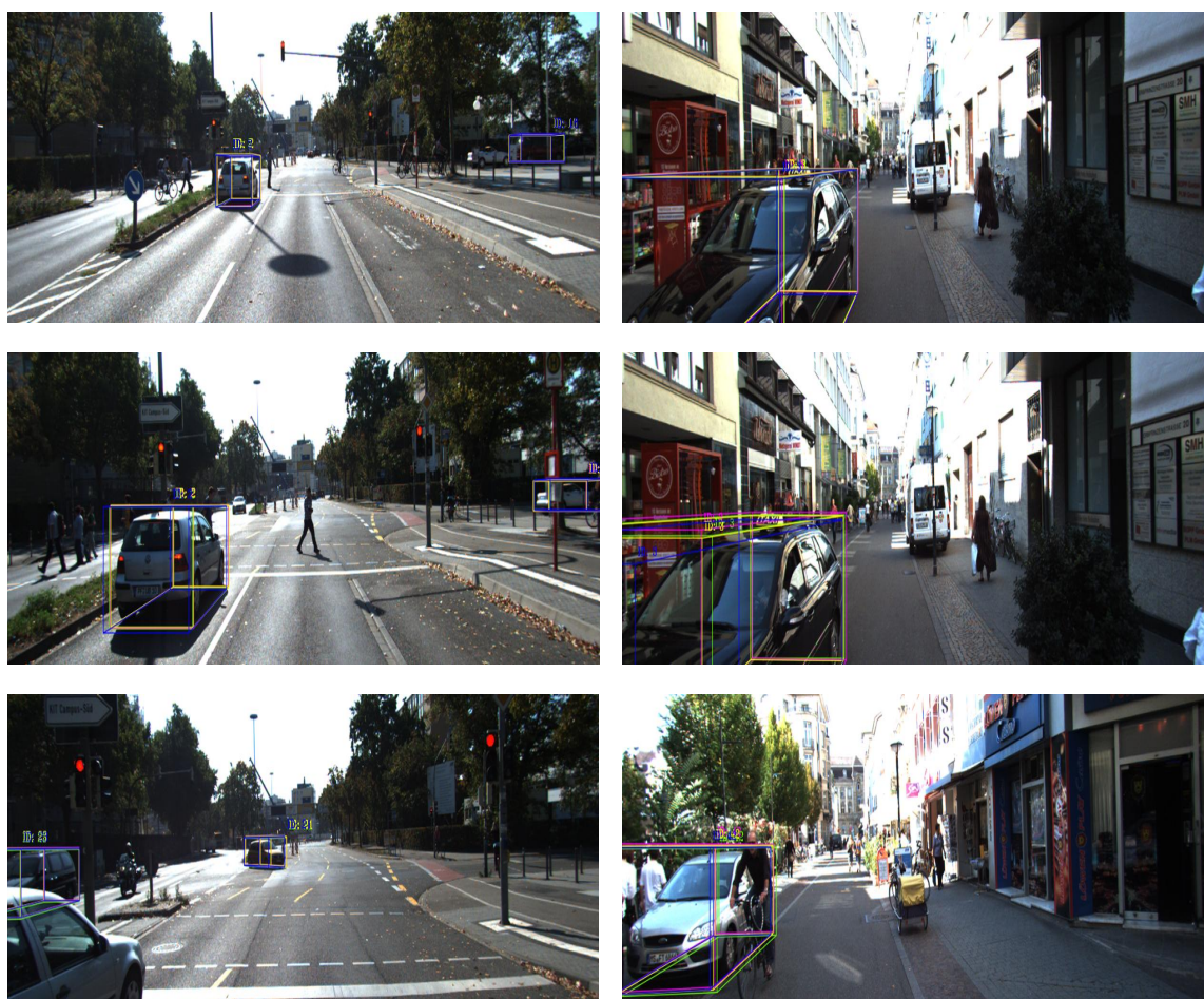
Figure 2. Qualitative comparison of different state estimators. Green, blue, red, and yellow bounding boxes represent ground truth, standard KF, KNet, and our method, respectively. As the estimator evolves from KF to our method, the estimated box aligns progressively closer to the ground truth.
