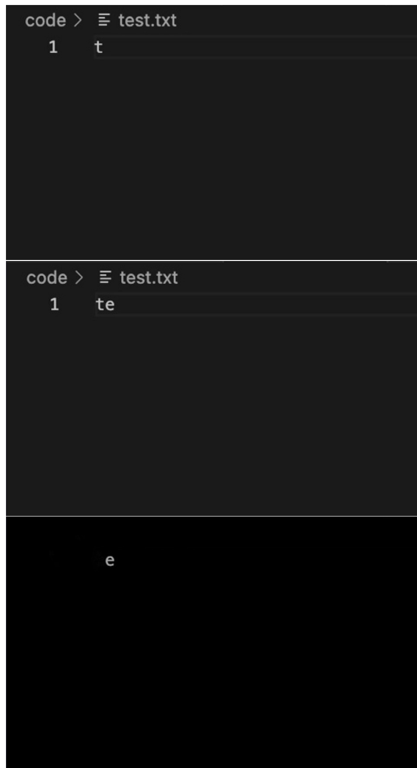
Figure 11. Frames before ( top ) and after ( centre ) a key press and their difference ( bottom ). The difference image highlights the newly typed character, enabling precise alignment between audio clicks and on-screen input.
