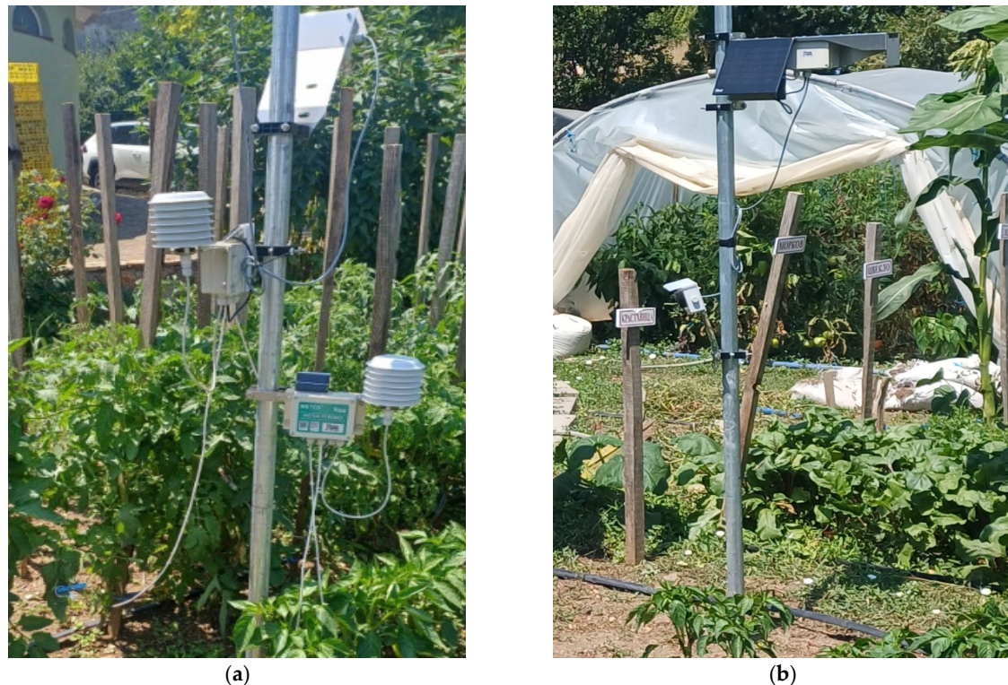
Figure 3. Experimental field deployment: (a) METOS STREMO environmental monitoring station; (b) autonomous wireless and solar-powered monitoring platform.
