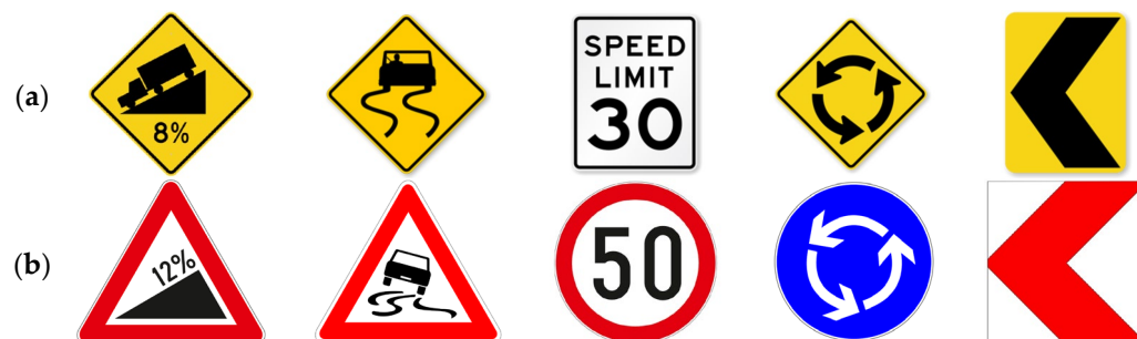
Figure 1. Comparison of road sign designs from (a) the United States (MUTCD system) and (b) Croatia (Vienna Convention-based system).
