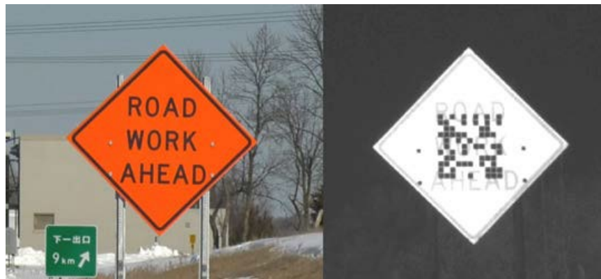
Figure 3. Example of visible and near-IR view of QR code (Source: [14]).
