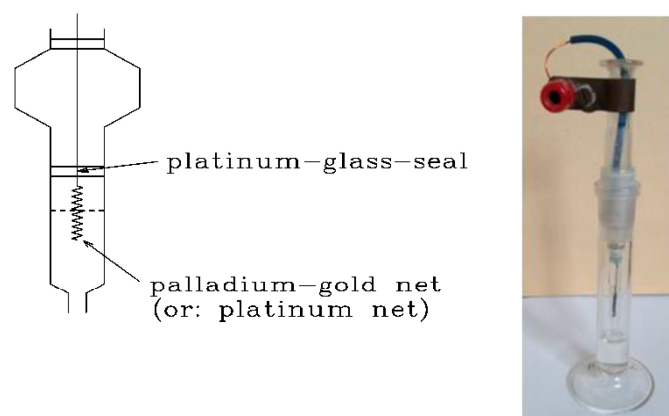
Figure 3. Schematic cross-section ( left ) and practical sample of an RHE according to Will.
