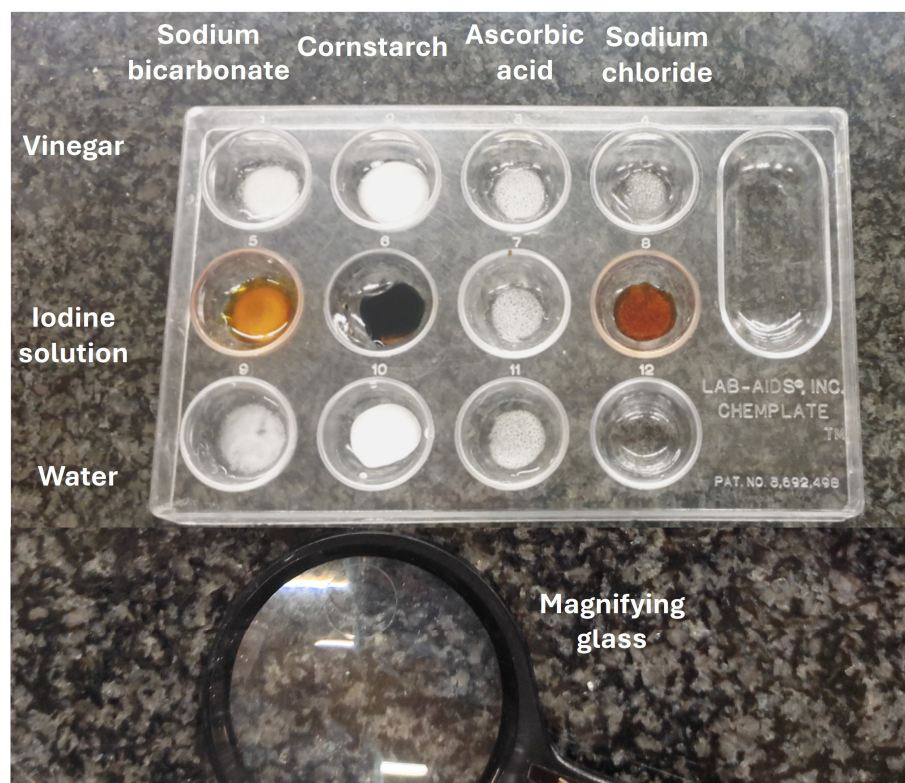
Figure 5. Mystery powder investigation. Diagnostic reactions of four known white solids—sodium bicarbonate, cornstarch, ascorbic acid, and sodium chloride—are compared with those of an unknown sample.
