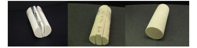
**Figure 4.** Three different core configurations were applied in this study. The fractured design was applied to maximize and provide constant reaction interface while maintaining flow conditions. A double-spacer design was applied to address limitations in diffusion length, while the non-fractured sample was used for more realistic scenarios.
