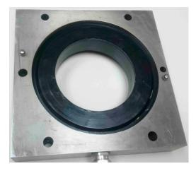
Figure 7. Center plate with the stator ring.
