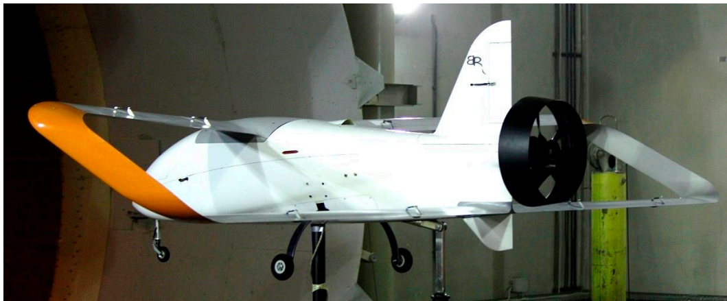
Figure 21. The airplane with ducted fan propulsion (photo took by Krzysztof Bogdański).
