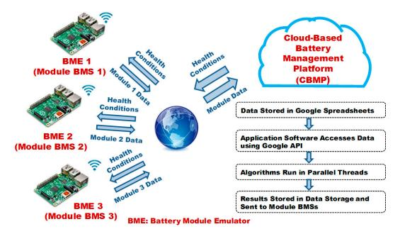
Figure 7. A Small-scale cloud-based BMS simulator.
