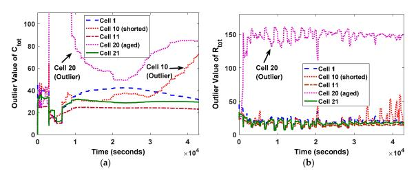
**Figure 9.** Outlier values of the total capacities and resistances of Cell 1, Cell 10 (internal short), Cell 11, Cell 20 (aged), and Cell 21 from the proposed outlier detection-based fault diagnosis algorithm in Google cloud: (a)  $O(Z_1)$  and (b)  $O(Z_2)$ .
