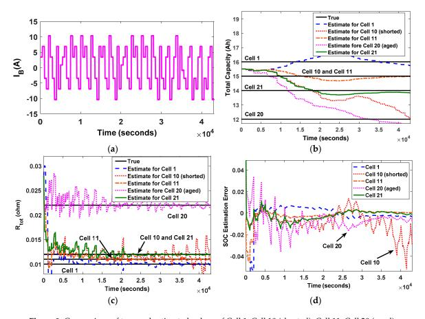
**Figure 8.** Comparison of true and estimated values of Cell 1, Cell 10 (shorted), Cell 11, Cell 20 (aged), and Cell 21 from the condition monitoring in Google cloud: (a) input current profile; (b)  $C_{tot}$ ; (c)  $R_{tot}$ ; and (d) state of charge (SOC) estimation error.
