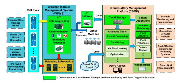
**Figure 2.** The system architecture of the proposed cyber-physical battery management system for the large-scale Li-ion battery energy storage systems and components of the proposed cloud-based battery condition monitoring and fault diagnosis platform.
