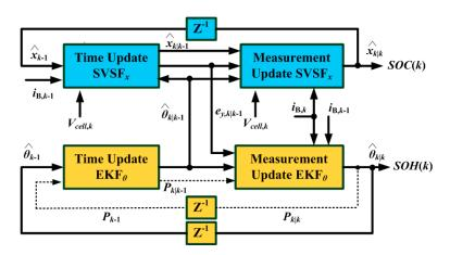
Figure 5. Block diagram of the hybrid filter.
