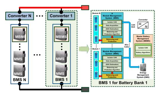
**Figure 1.** The conventional battery management systems (BMSs) where each BMS consists of module management systems (MMSs) and a master BMS for a large-scale Li-ion battery energy storage system (BESS).
