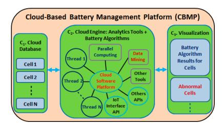
Figure 3. The proposed cloud battery management system platform.
