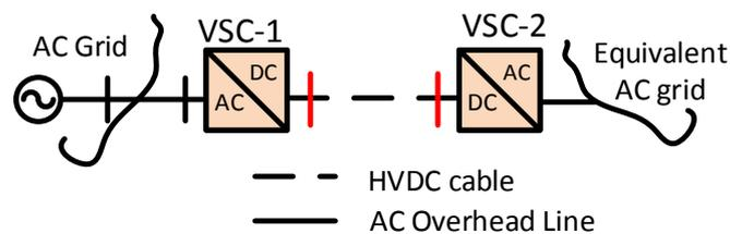
Figure 1. HVDC (High voltage direct current) point-to-point link.
