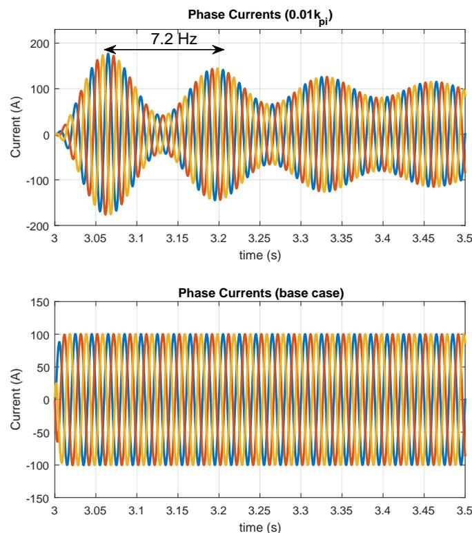
**Figure 12.** (Top plot) time domain plot of phase currents in  $abc$  frame, showing sustained resonances for the case with  $0.01 \times k_{pi}$  with a matching frequency with that of frequency response; (Bottom plot) base case with no resonance.
