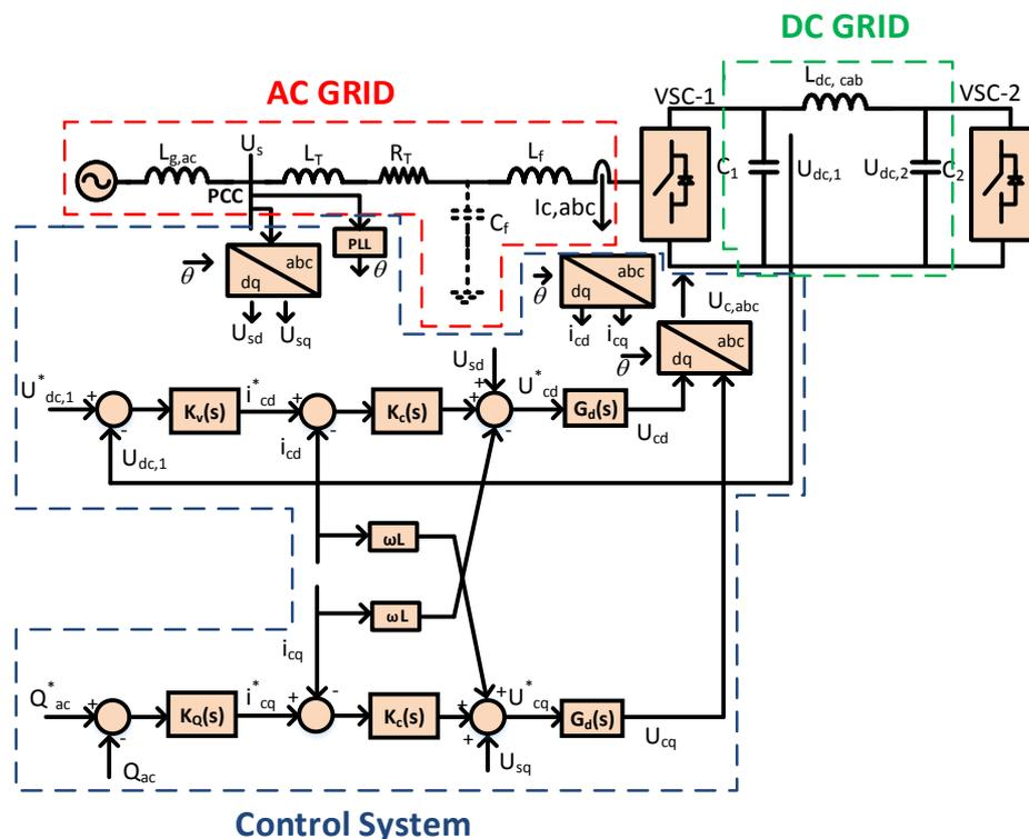
Figure 2. HVDC impedance circuit and control architecture.
