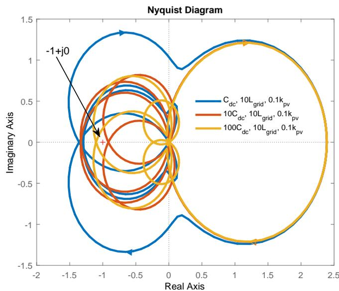
Figure 28. Stability sensitivity to varying DC grid capacitance.
