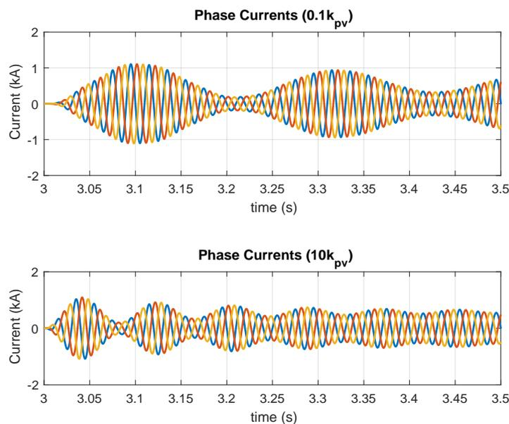
**Figure 22.** (Top plot) time domain plot of Phase AC currents in the abc frame for the case of  $0.1k_{pv}$ ; (Bottom plot) case of  $10k_{pv}$ .
