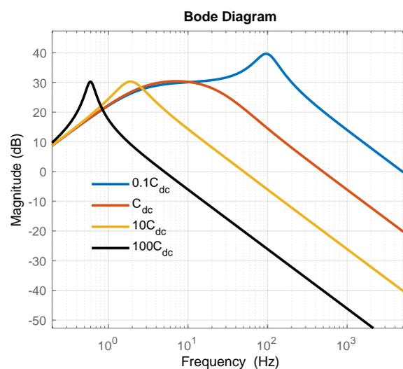
**Figure 24.** Input impedance sensitivity to total DC capacitance with capacitances  $0.1\times$ ,  $1\times$ ,  $10\times$ ,  $100\times C_{DC,bus}$  at both terminals, where  $C_{DC,bus}$  is the nominal bus capacitance of  $300\ \mu\text{F}$ .
