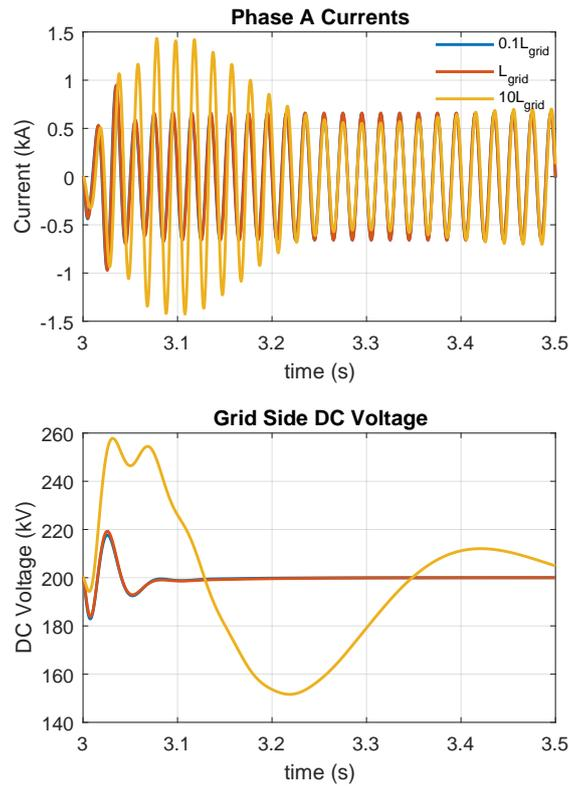
Figure 27. (Top) Phase A currents for varying SCRs; (Bottom) grid side DC voltages for varying SCRs.
