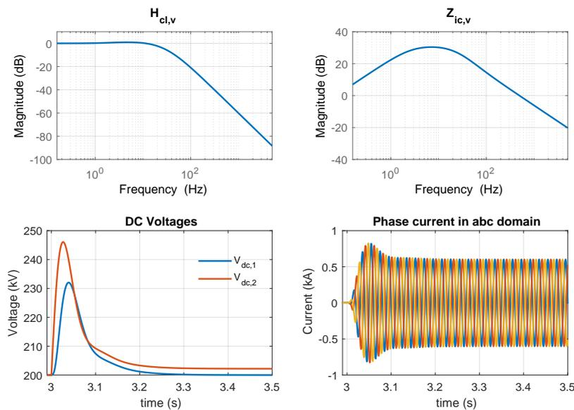
**Figure 8.** (Top left) Frequency response of closed-loop output to reference transfer function; (Top right) frequency response of input impedance from DC (base case); (Bottom left) time response of DC voltages; (Bottom right) time response plot of phase currents in abc domain.
