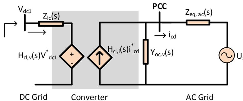
Figure 10. Impedance model of converter and connected grid impedance.
