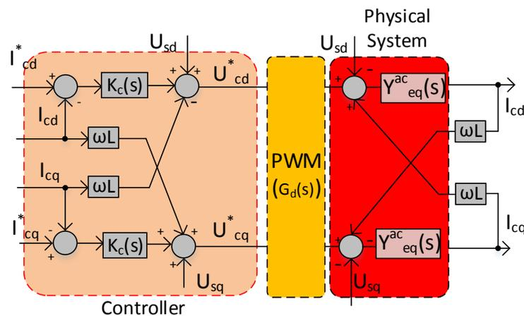
Figure 3. Inner current loop and physical grid.
