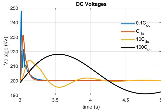
Figure 25. Time domain plot of grid side DC voltage varying DC capacitance.
