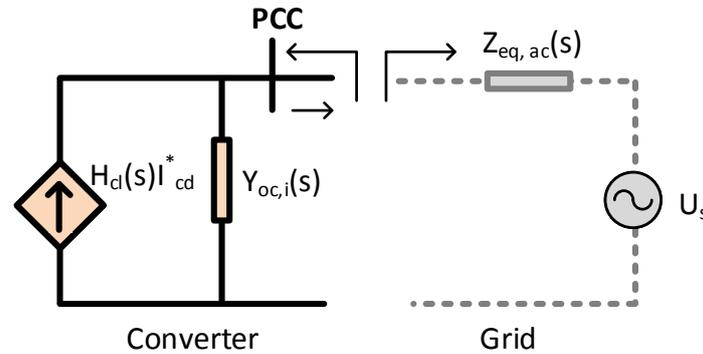
Figure 5. Equivalent circuit representation of current controller relative to the grid.
