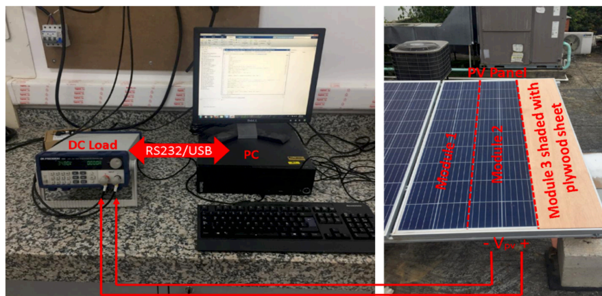
Figure 11. Experimental platform. Left: electronic load and PC in the laboratory. Right: PV module and piece of wood in the roof. Red lines from right to left represent the electrical connection between the module an the electronic load.
