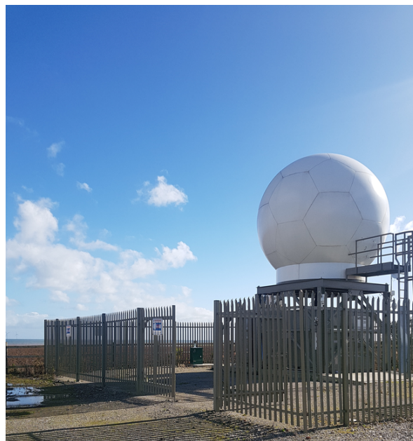
Figure 6. One of the two Doppler radar units deployed for the BEACon project [59,62].
