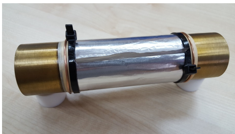
Figure 2. A photograph of the insulation sample prepared for testing.
