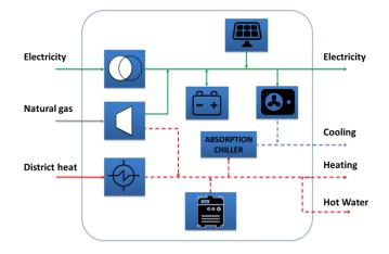
Figure 1. An energy hub containing typical elements.
