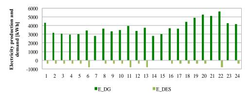
**Figure 10.** Optimal daily schedule of diesel generators and desalination units in January (average load month) in the TO-BE scenario 1. In this figure E\_DG is the variable  $E_{DG}$  and E\_DES is the variable  $E_{DES}$ .
