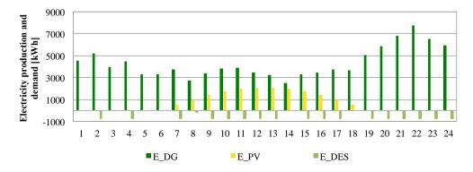
**Figure 18.** Optimal daily schedule of diesel generators and desalination units in August (maximum load month) in the TO-BE scenario 2. In this figure E\_DG is the variable  $E_{DG}$ , E\_PV is the variable  $E_{PV}$  and E\_DES is the variable  $E_{DES}$ .
