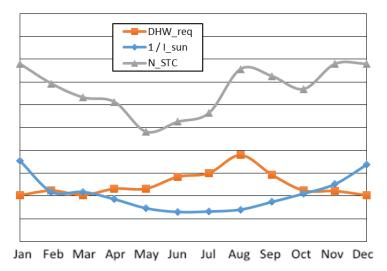
**Figure 15.** Solar thermal collectors STC size influence in monthly optimizations in the TO-BE scenario 2. In this figure DHW\_req is the variable  $DHW_{req}$ , I\_sun is the solar radiation and N\_STC is the variable  $N_{STC}$ .
