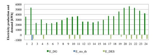
**Figure 17.** Optimal daily schedule of diesel generators and desalination units in January (average load month) in the TO-BE scenario 2. In this figure E\_DG is the variable  $E_{DG}$ , E\_sto\_th is the variable  $E_{sto,th}$  and E\_DES is the variable  $E_{DES}$ .
