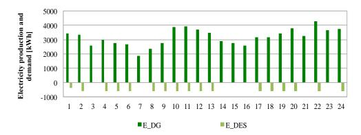
**Figure 9.** Optimal daily schedule of diesel generators and desalination units in May (minimum load month) in the TO-BE scenario 1. In this figure E\_DG is the variable  $E_{DG}$  and E\_DES is the variable  $E_{DES}$ .
