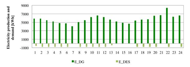
**Figure 11.** Optimal daily schedule of diesel generators and desalination units in August (maximum load month) in the TO-BE scenario 1. In this figure E\_DG is the variable  $E_{DG}$  and E\_DES is the variable  $E_{DES}$ .
