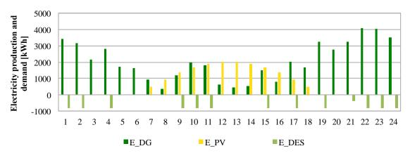
**Figure 16.** Optimal daily schedule of diesel generators and desalination units in May (minimum load month) in the TO-BE scenario 2. In this figure E\_DG is the variable  $E_{DG}$ , E\_PV is the variable  $E_{PV}$  and E\_DES is the variable  $E_{DES}$ .
