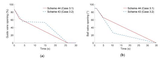
Figure 18. Comparison of optimized closing schemes in Case 3 for (a) guide vanes and (b) ball valve.
