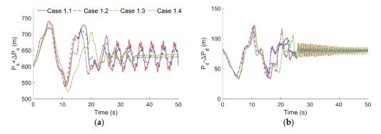
**Figure 14.** Comparison of dynamic pressure envelopes between subcases in Case 1 at (**a**) the spiral case and (**b**) the draft tube.
