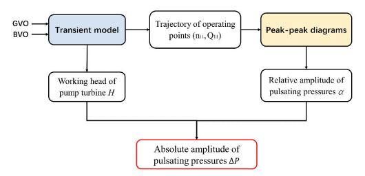
Figure 6. Process of pulsating pressure estimation.
