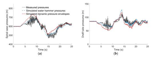
Figure 10. Comparison of measured and simulated pressures at (a) spiral case and (b) draft tube.
