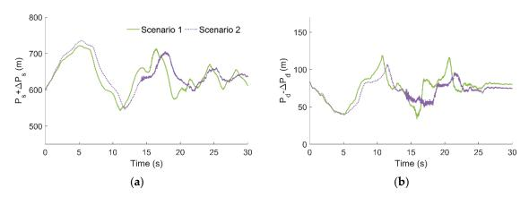
**Figure 16.** Comparison of dynamic pressure envelopes between the two scenarios in Case 2 at (a) the spiral case and (b) the draft tube.
