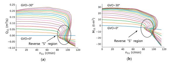
Figure 3. Characteristic curves of pump turbine: (a) flow-speed and (b) torque-speed.
