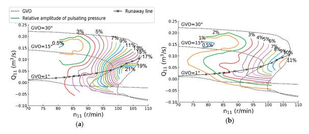
**Figure 5.** Extended peak-to-peak diagrams of the pulsating pressures in a model pump turbine at (a) the spiral case and (b) the draft tube.
