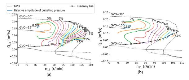
**Figure 4.** Peak-to-peak diagrams of pulsating pressures in a model pump turbine at (**a**) the spiral case and (**b**) the draft tube.
