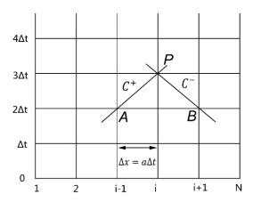
Figure 2. Difference mesh for the method of characteristic.
