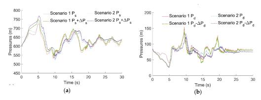
**Figure 19.** Comparison of water hammer pressure and dynamic pressure envelopes between two scenarios in Case 3.1: (a) at spiral case and (b) at draft tube.
