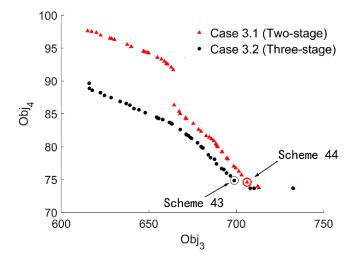
Figure 17. Pareto fronts obtained by different guide vane closing schemes in Case 3.
