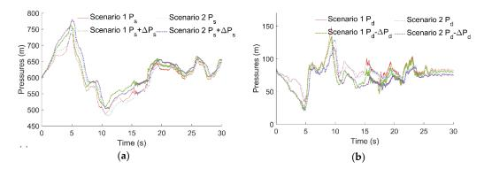
**Figure 20.** Comparison of water hammer pressure and dynamic pressure envelopes between two scenarios in Case 3.2: (a) at spiral case and (b) at draft tube.
