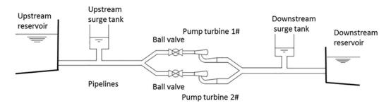
**Figure 1.** Basic configuration of a pumped-storage plant (PSP) with two pump turbines sharing the same main pipelines.
