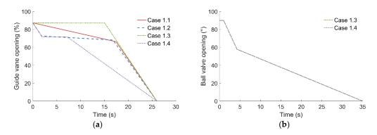
Figure 12. Optimized closing schemes in Case 1 for (a) guide vanes and (b) ball valve.
