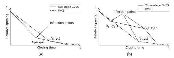
**Figure 7.** Closing operation of a PSP with (**a**) a two-stage guide vane closing scheme (GVCS) and (**b**) a three-stage GVCS.
