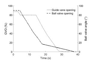
Figure 8. GVCS and ball valve closing schemes (BVCS) in the field test.
