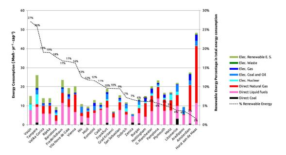
**Figure 5.** Energy consumption by fuel within the direct and indirect (in electric vector) energy consumptions by municipality (note that the total consumption of cities obtained from mPOWER survey differs, as shown in Figure 3, from the national average data provided by International Energy Agency (IEA)).
