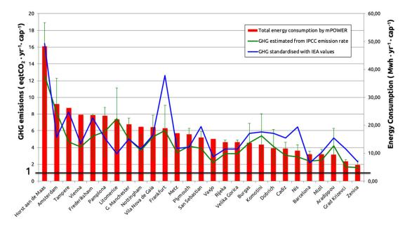
**Figure 7.** Energy consumption per capita by municipality, and the respective greenhouse gas (GHG) emissions obtained from the survey (IEA standardised) and calculated from the energy consumption and the IPCC emission intensities.
