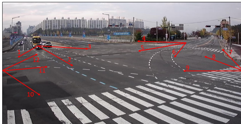
Figure 1. An example of a complex intersection with 12 movements with a single view of the CCTV.
