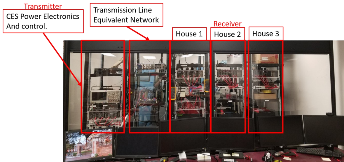
Figure 7. Live-scale DC microgrid physical setup.
