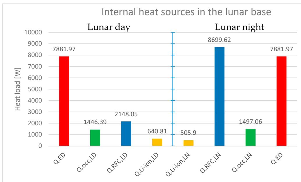
**Figure 5.** Internal heat loads in the lunar base during the lunar cycle.
