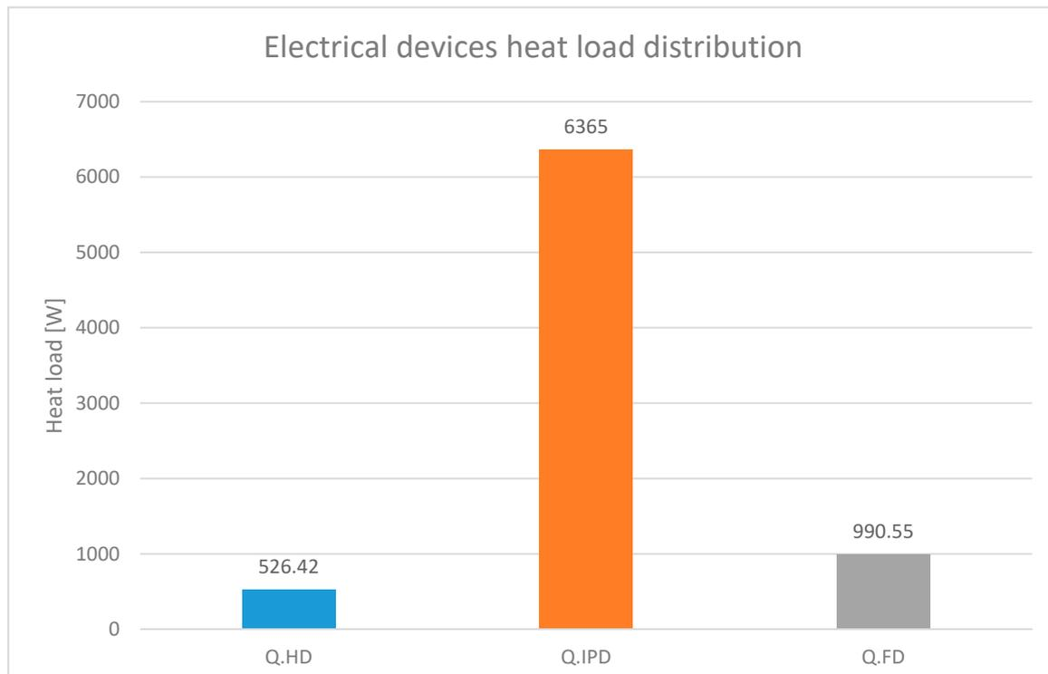
**Figure 6.** Nominal operations heat load distribution for the three categories of electrical devices.
