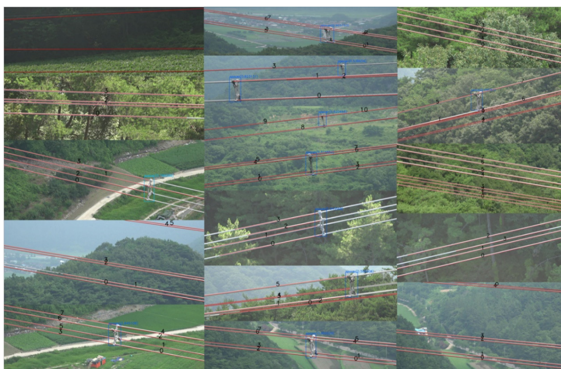
Figure 5. Power line detection results. The proposed power line detection algorithm shows robustness against cluttered background and different lighting conditions (here detected power lines are marked with red color, and labelled with an ID number).
