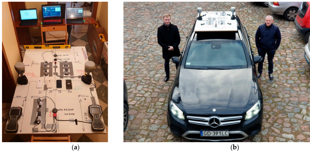
Figure 4. Testing electrical connections of the measurement equipment (a) and a plate with measurement equipment assembled on a passenger car (b).
