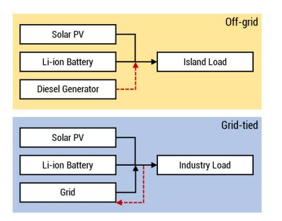
Figure 2. Architecture of the hybrid off-grid (top) and grid-tied (bottom) energy systems.
