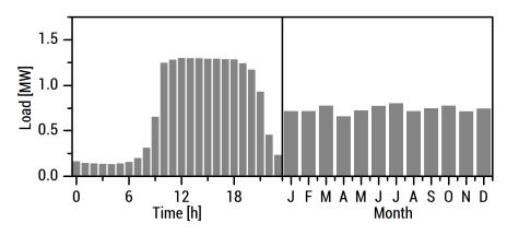
Figure A4. Hourly (left) and monthly (right) average load consumption in the commercial mall.
