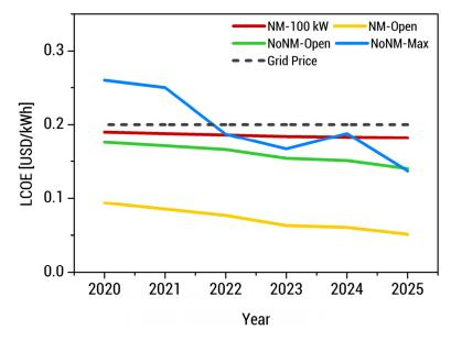
**Figure 7.** Calculated future LCOE of different grid-tied scenarios in comparison with the average annual cost of electricity from the grid within the analysis period of 2020 to 2025. The NoNM-Open scenario is the least-cost scenario allowed by current Philippine policies.
