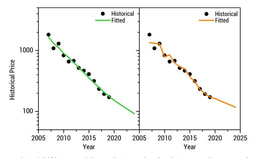
**Figure 5.** Li-ion NMC battery pack historical prices and predicted prices according to a two-factor (**left**) and four-factor (**right**) learning curve model. The two-factor model falls below the 100 USD/kWh price point in agreement with expert predictions. The four-factor model is overfitted and may lead to inaccurate results.
