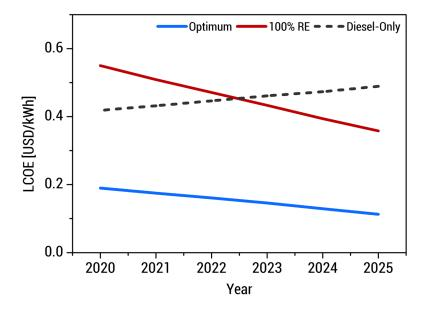
**Figure 6.** Calculated future LCOE of the optimum system and 100% RE system in comparison with the TCGR within the analysis period of 2020 to 2025. The LCOE of the optimum system is already lower than the diesel-only system in 2020, while the 100% RE system yields a lower LCOE than the diesel-only system in 2023.
