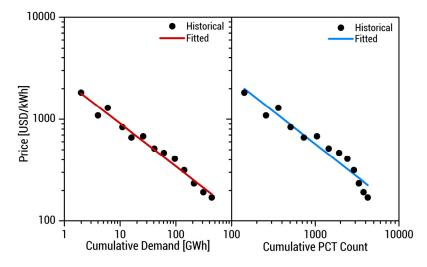
**Figure 3.** Learning rates using the single-factor learning curve model for Li-ion NMC battery storage. The figure shows learning by using (**left**) and learning by innovation (**right**).
