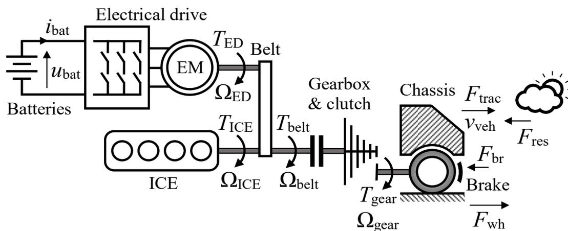
Figure 1. Studied system: a parallel hybrid truck.
