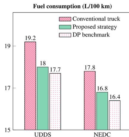
Figure 6. Comparison of fuel consumptions via simulation.
