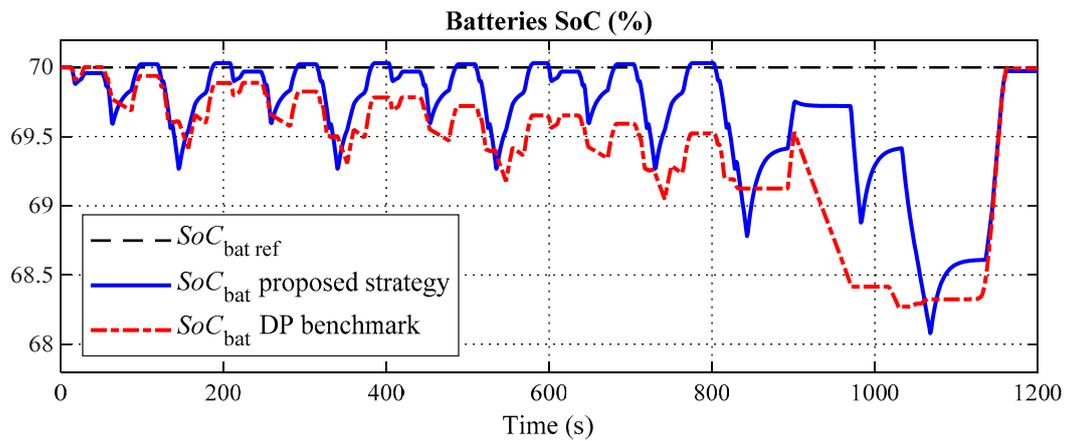
Figure 9. (Simulation) batteries SoC evolutions with NEDC.
