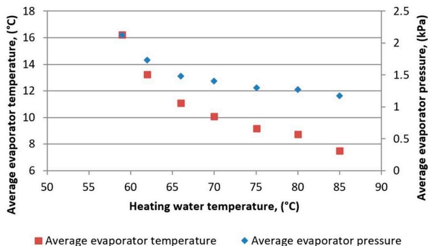
Figure 6. The influence of the heating water temperature on the average evaporator temperature and the average evaporator pressure.
