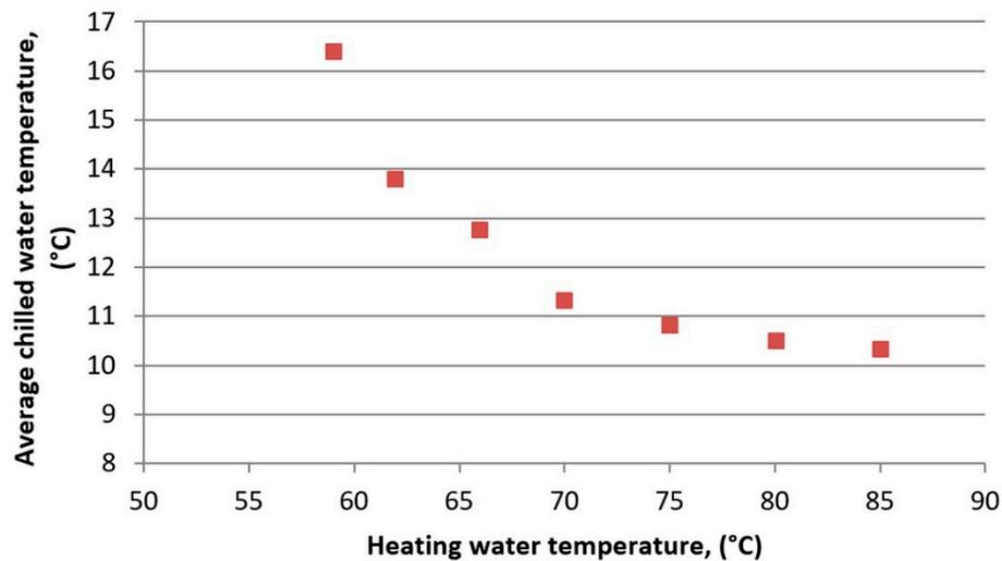
Figure 5. The influence of the heating water temperature on the average chilled water temperature.
