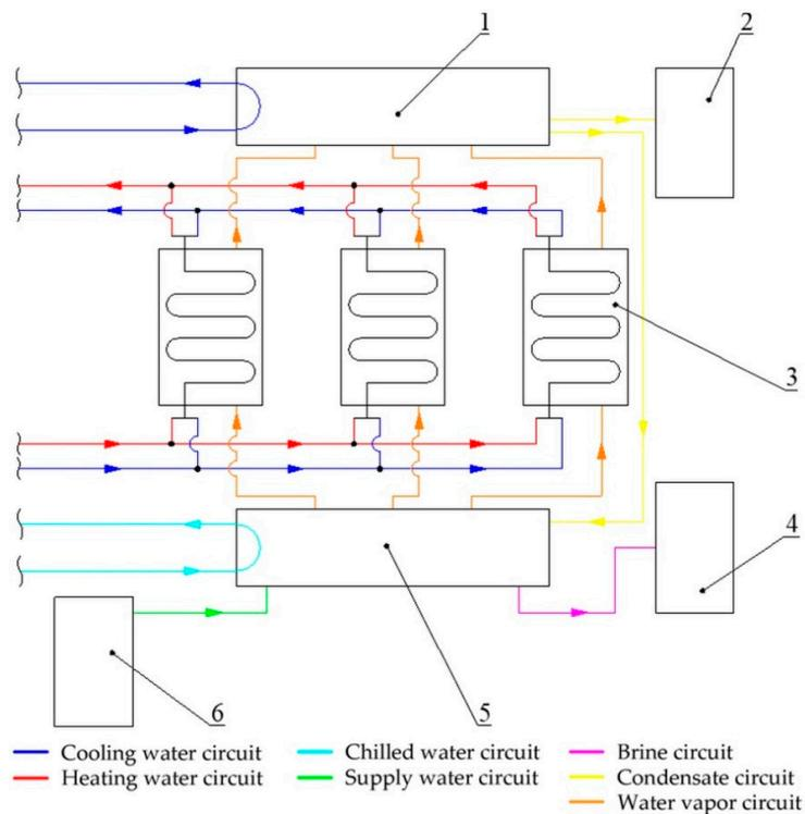
**Figure 1.** The simplified diagram of the investigated adsorption chiller with desalination function. 1—condenser; 2—distillate tank; 3—adsorbent bed; 4—brine tank; 5—evaporator; 6—deaerator.
