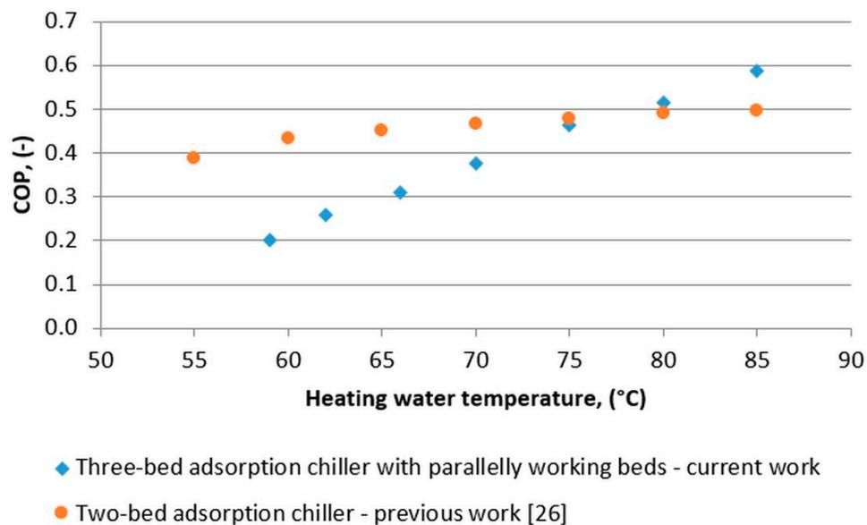
**Figure 3.** The influence of the heating water temperature on the coefficient of performance (COP).
