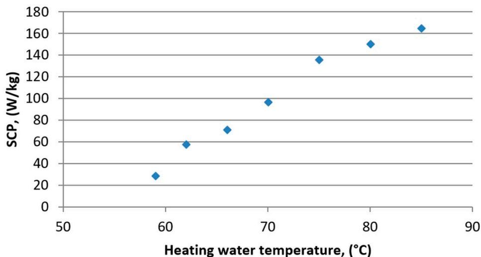
**Figure 4.** The influence of the heating water temperature on the specific cooling power (SCP).
