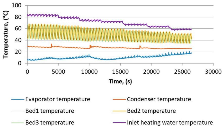
**Figure 7.** The changes in the evaporator, condenser, and bed temperatures in the function of time.
