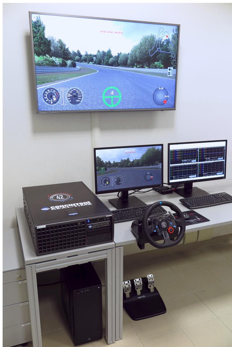
Figure 7. Hardware-in-the-loop real-time car simulator.
