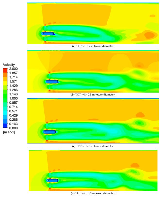
Figure 9. Velocity contour of the water for different tower diameter in the Z-X plane.
