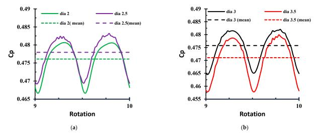
Figure 5. Coefficient of performance for tower having diameter (a) 2 and 2.5 m (b) 3 and 3.5 m.
