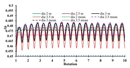
Figure 4. Coefficient of performance for different tower diameter for 10 rotations.
