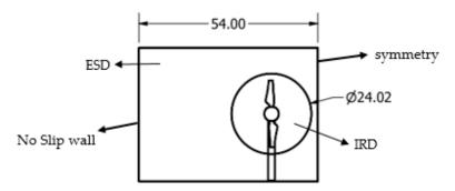
**Figure 2.** Front view of computational domain with External Stationary and Internal Rotating Domain.
