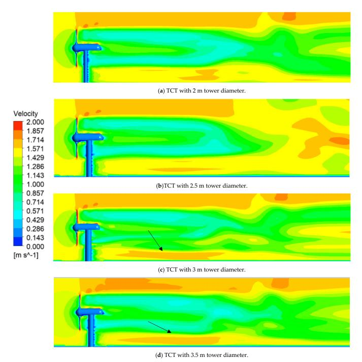
**Figure 8.** Velocity contour of the water in X-Y plane throughout the domain.
