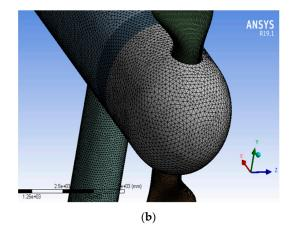
Figure 1. (a) Mesh detail of external and internal rotating domain (b) mesh of turbine.
