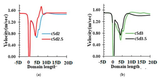
**Figure 7.** Velocity contour of the water throughout the domain at the center line of the turbine (a) TCT with tower 2, 2.5 m diameter (b) TCT with tower 3 and 3.5 m diameter.
