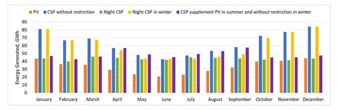
Figure 8. Annual energy generation for each plant according to the month of the year (CSP with 13 h of storage).
