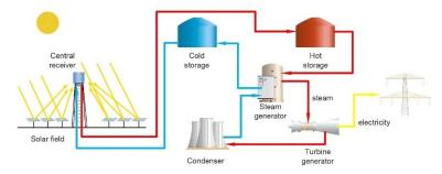
Figure 2. Schematic of a tower CSP generation system.
