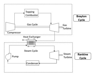
**Figure 3.** Scheme of a combined cycle power plant. A Brayton cycle is shown above, and the cycle below corresponds to a Rankine Cycle.
