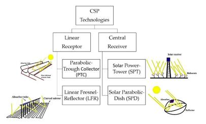
**Figure 1.** Classification of existing concentrated solar power (CSP) technologies. Source of the images [17].
